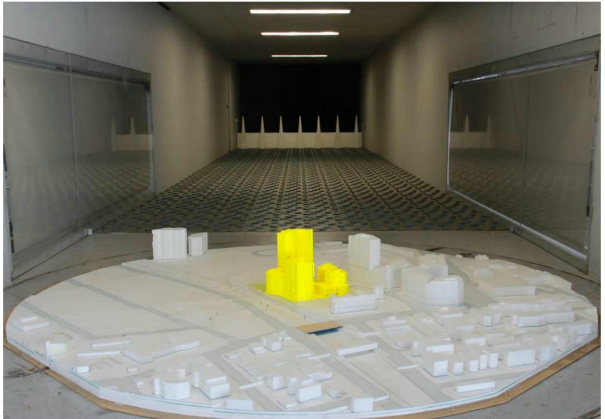
Figure 3b: Photograph of the Wind Tunnel Model (view from the south-east)
